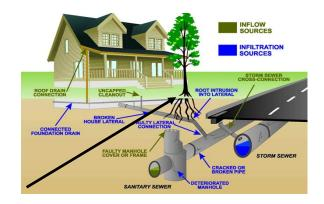
Plant roots are another frequent cause of sewer backups and overflows. The roots of shrubs and trees naturally seek any water source. The roots probe the sewer line seeking any opening, such as a crack or a poorly sealed joint. Once the sewer line is penetrated, the roots form a ball and block the line.
